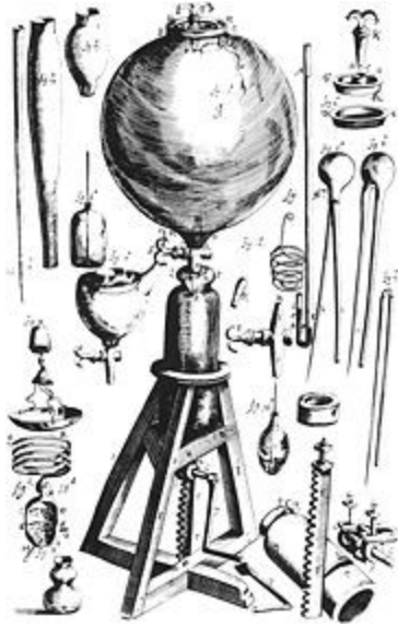
Drawing of Robert Boyle 's air pump (1661). From New Experiments ... Touching the Spring of the Air ... Public Domain.
